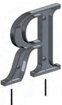
3C - Bottom or Top Stud Add 15% to brushed letter price. Letters 4"-30", Minimum 3/8" thick Letters over 12" may require tie-back (not supplied).
