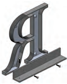
3D - Bottom Back Angle Bracket Mount Add 35% to brushed letter price. Letters 4"-30", Minimum 3/8" thick. Letters over 12" may require tie-back (not supplied). Aluminum angle is 2" x 2" with a painted finish.
