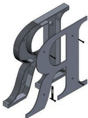
Bottom Stud w/Back Multiply the brushed letter price by 2 Letters 4"-24", Minimum 3/8" thick Includes painted or anodized 1/8" thick aluminum back. Letters over 8" may require tie-back (not supplied). Can be full cover or inset for flush edge.
